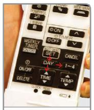
The buttons on the remote controller are set out in the order of how you set the timer. The clock on the remote must be set to the correct time.
